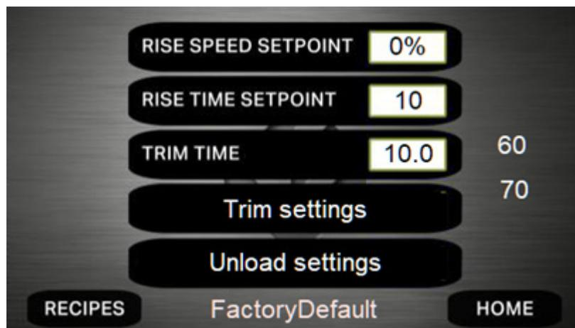
6. This screen will allow you to program every part of the cycle individually. Rise Speed setpoint (1-100%) controls how fast the **Rise Conveyor** runs at.
